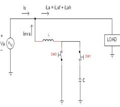
Fig.2 Single Phase Equivalent Circuit of the system and VSI
